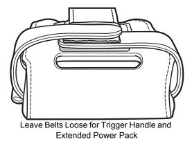
Insert the device into the holster with the device exit window facing up and the display against the body.
