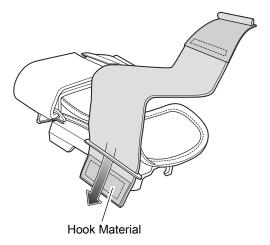
Figure 117 Feed Strap through Rear Slots
