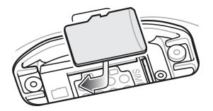
10. Push the microSD card into the SD card slot.
