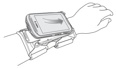
2. Rotate the bottom of the device into the mount and snap into place.
