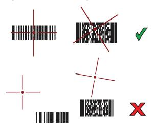
Figure 76 RS6000 Pick List Mode with Multiple Barcodes in Aiming Pattern
