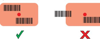
Figure 73 SE4710 Aiming Pattern with Multiple Barcodes
