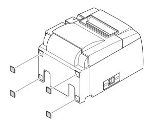
Attach the four rubber feet in the positions shown in the figure.
