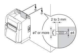
(2) Position the printer over the screws, etc., on the wall and then slide it downward to set it in place.
