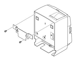
(1) Attach the holding plate to the printer. Then tighten the two screws that were supplied to secure it in place.
